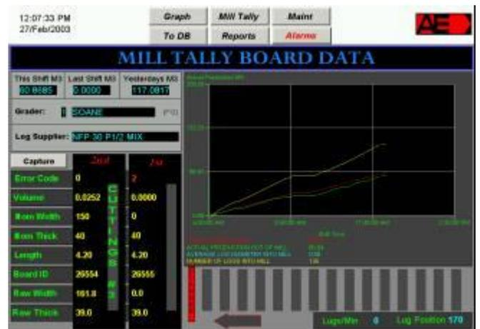
The Mill View™ management reporting system can be configured on various SCADA platforms inc iFix , RSView ,Wonderware and is customized to the clients requirements .
